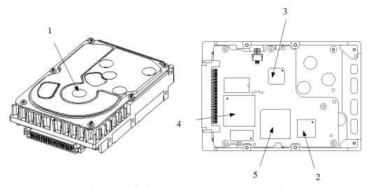
Figure 4.6 Surface temperature measurement points
